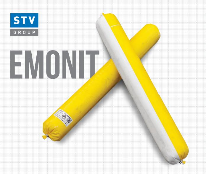
Emonit is an industrial emulsion explosive of mucky consistency and yellowish to brown color. Emonit is an emulsion matrix and a nitroglycerin / nitroglycol sensitizer mixed so that the resulting product has the specified functional properties. The bulk mixture is loaded into PE foil of Ø 65 mm and larger. The minimum cartridge weight is 2000 grams.
