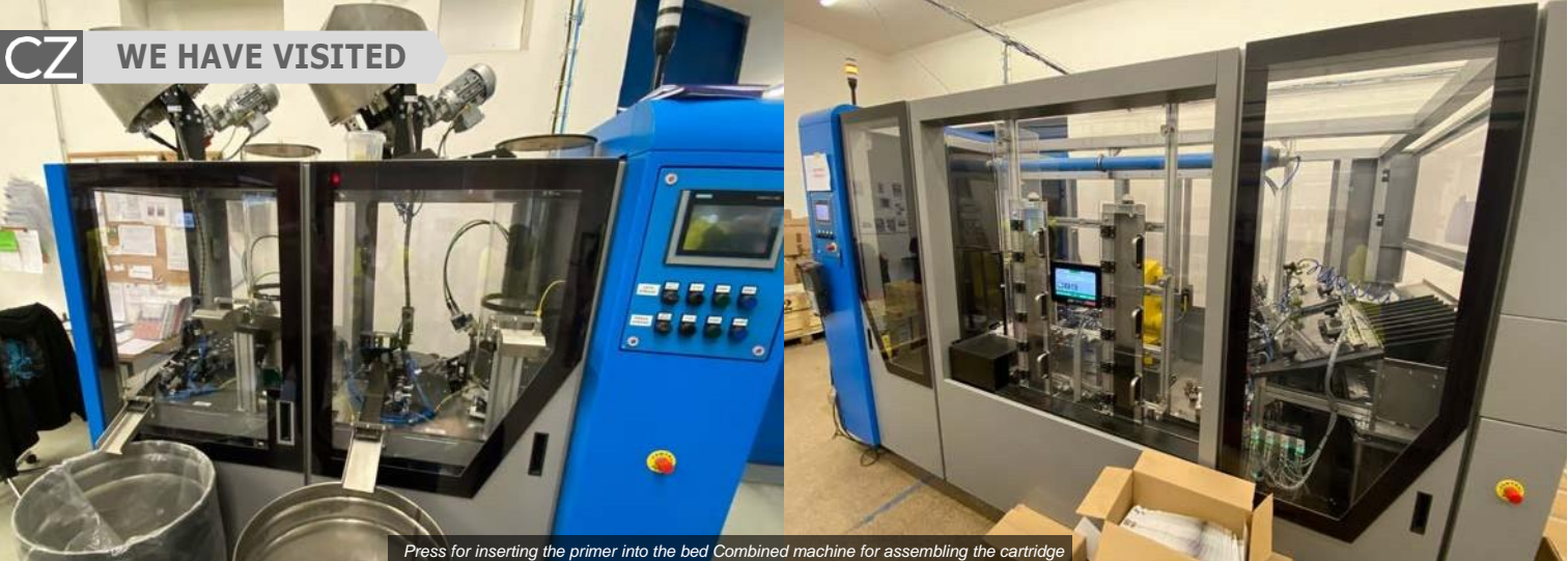
Press for inserting the primer into the bed Combined machine for assembling the cartridge
