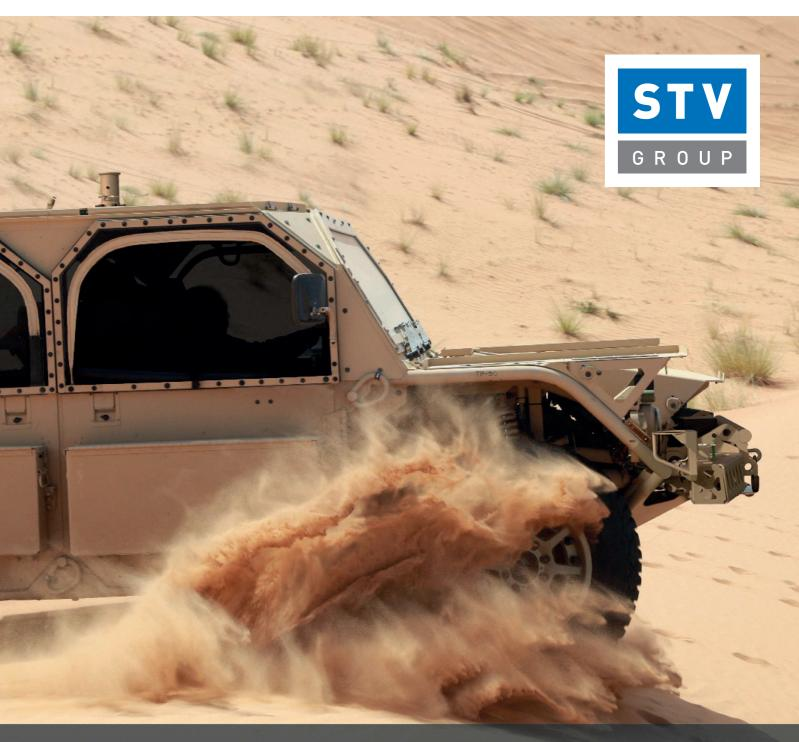
The Flyer® 72 - Heavy Duty (F72-HD) ground mobility vehicle is a non-developmental item, purpose-built, lightweight vehicle designed to meet complex mission sets. Selected by the U.S. Special Operations Command (USSOCOM) as the vehicle of choice for their Ground Mobility 1.1 (GMV 1.1) program, at 72" wide it is capable of internal transport in the CH-47 and C-130 aircraft.
